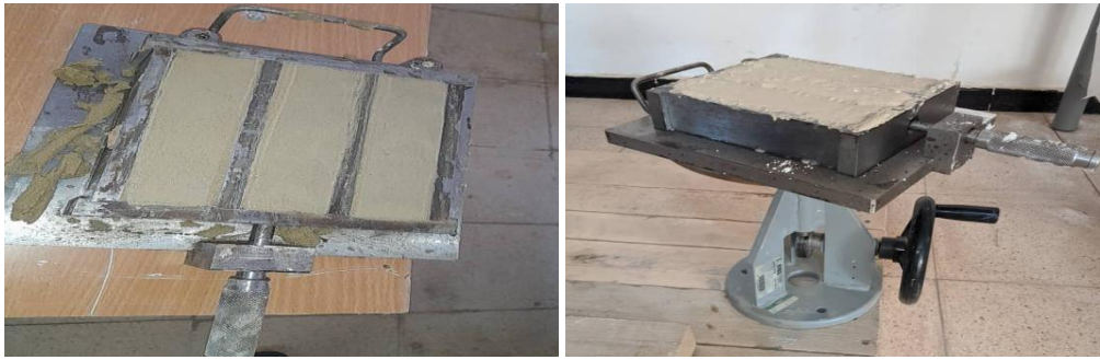
Figure III.4 : Compactages des moules en pate ciment/diatomite.
