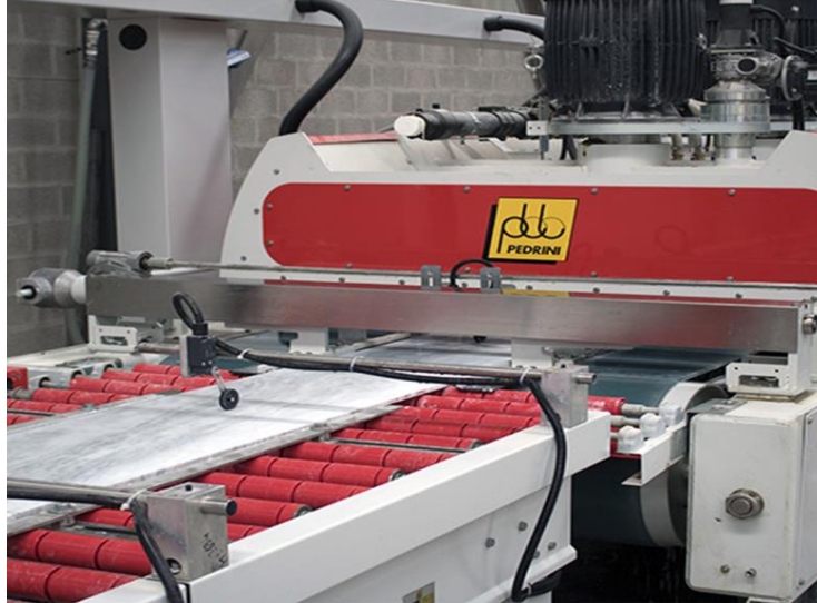
Figure II. 8 : Machine de Finition [19].
