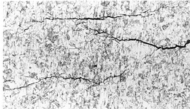
Figure I.7 : Corrosion inter granulaire [32].
