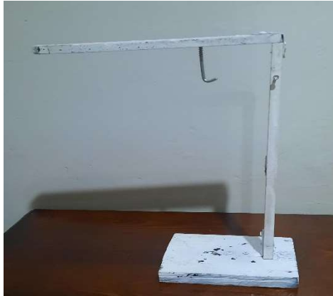
figure 3.46 : Photo of the handcrafted wooden arm supporting the test rig
