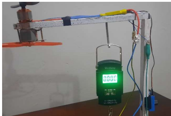
figure 3.55 : Image of the digital scale placed under the wooden arm to measure thrust
