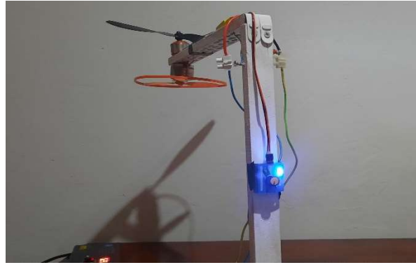
figure 3.52 : Close-up of the servo tester connected to the ESC
