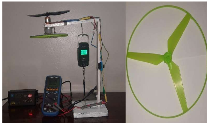
figure 3.63 : Photo showing the generator with the large 3-blade propeller installed
