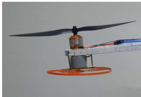
figure 3.49 : Image showing the small wind generator fixed beside the airflow path
