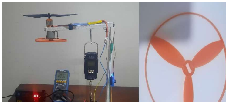
figure 3.61 : Photo of the generator with the small 3-blade propeller installed
