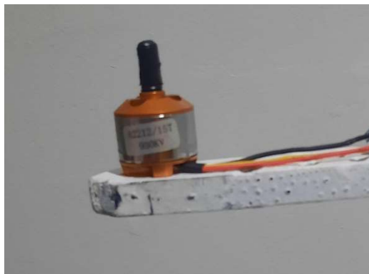
figure 3.47 : Close-up image of the mounted 2212A 15T 930KV motor
