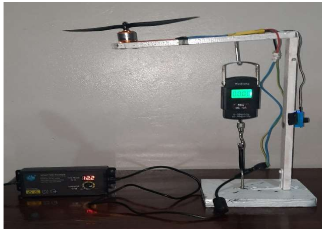
figure 3.57 : Photo of the test setup without the generator, showing only the motor and propeller
