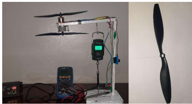
figure 3.59 : Photo of the full setup with generator and 1045 propeller installed
