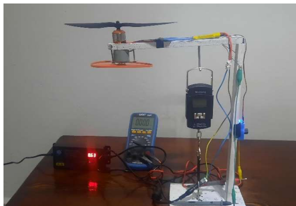
figure 3.56 : Illustration showing the complete single-arm test rig with all components installed
