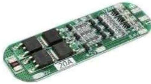
figure 3.38 : Battery Management System (BMS)
