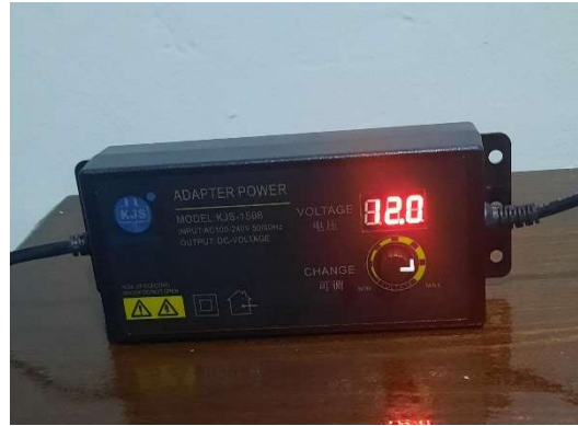
figure 3.50 : Photo of the power supply unit used in the experiment
