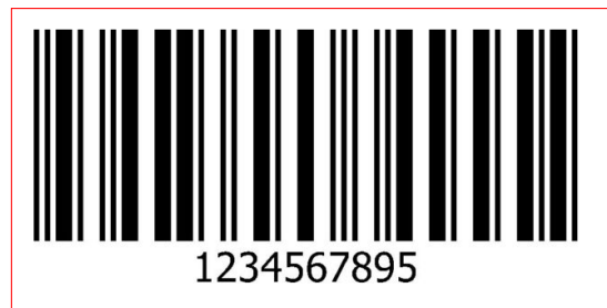
Figure 2.2: Codabar encoding for digits 0 to 9
