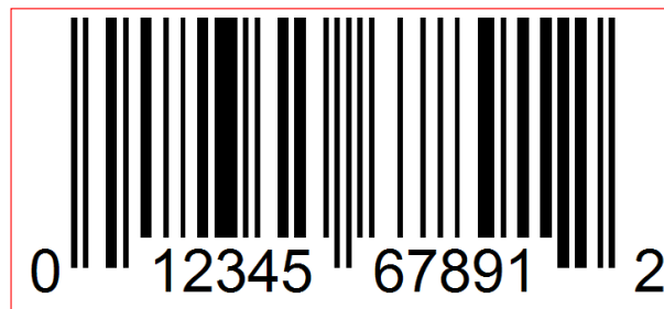
Figure 2.5: UPC coding for 012345678912
